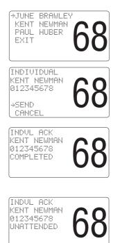
**Note:** If there is not any data registered in the directory you cannot proceed to the 3rd step. See the SETUP section for directory setup instructions. Select an open (unused) working channel first, then make the call. After the acknowledgment, both radios tune to the previously selected channel.
