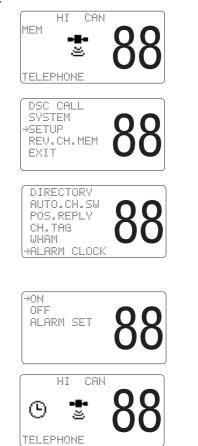
**Note:** The alarm sounds when the set time is reached, you can turn the alarm Off by pressing any key. Alarm mode will turn Off automatically once the alarm sounds.
